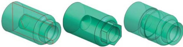
Turning > Milling > Turning
