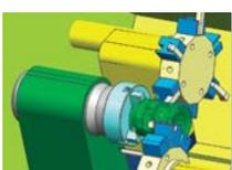
**Machining simulation** – to avoid tying up a machine in unproductive prove-outs, the integrated machine tool simulation provides a more complete simulation than most systems with its machine code driven motion.
