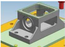
**2 1/2- Axis milling** – 2 1/2-Axis roughing patterns can be applied based on basic boundary data or solid geometry. Zig-zag, offset, and plunge milling are examples of the toolpaths provided. High-speed roughing toolpaths such as trochoidal are available here. Feature based machining functions automate the identification and programming of slots and faces.
