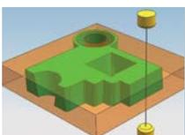
**Wire EDM** – a complete solution for programming 2 4-Axis wire EDM machines. A range of wire operations is available, including multi-pass profiling, wire reversing and area removal.
