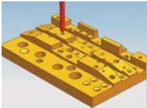
**Drilling** – addresses drilling, reaming, boring, tapping, peck drilling, and custom cycles. Automated hole making is available with the feature based machining options.
