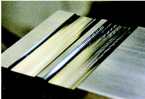
Figure 1: Two cuts showing stable and chatter machining conditions.
