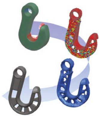
Topology optimization for new crane hook design
