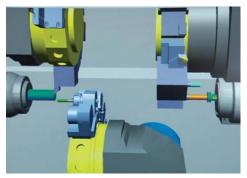
Virtual environment for machine tool setup work.
