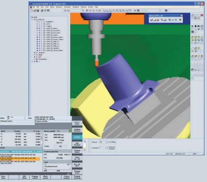
Siemens Virtual Machine uses the core software from the real Sinumerik controller to drive the machine simulation and provide the simulated user interface.
