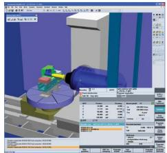
You can program Virtual Machine using the same control panel software on the PC as the real machine.
