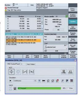
The Sinumerik display panel view in Virtual Machine makes it ideal for use by the machine operator.
