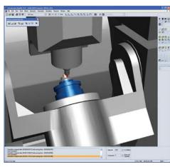
Virtual Machine reads and reacts to Sinumerik code just like the real 840D controller.
