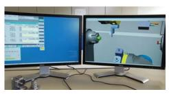
You can validate NC programs on a virtual machine tool.
