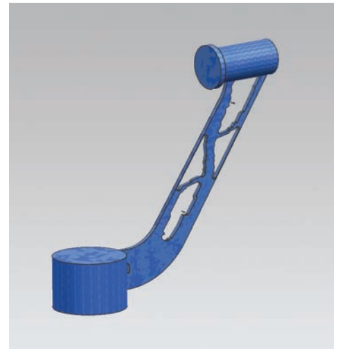
Smoothed surfaces from conceptual optimization that designers can use as starting point for design.
