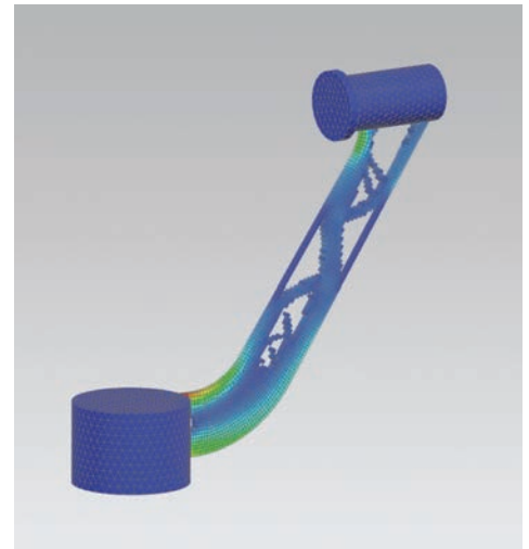
Optimized concept with stress results.
