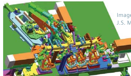
Welding fixture complete with clamps and welding guns for an automotive assembly.
