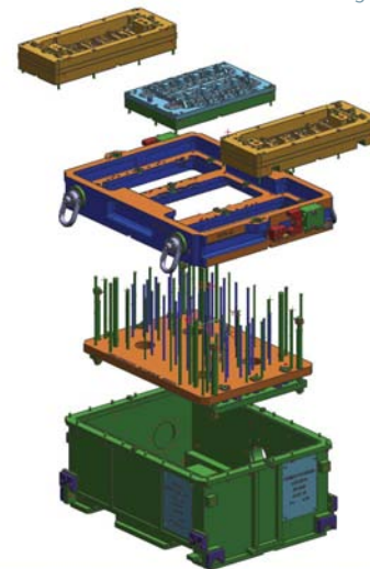
NX models of sand casting molds and associated equipment for automotive engine components.
