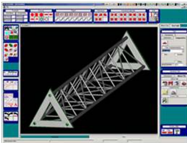
Designing and assembling a tube based structure prior to manufacture using Adige's machine tools
