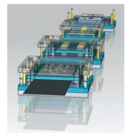
Material transfer equipment can be added from a library. Motion simulation is used to verify that the part transfer and die sequencing perform correctly. Automatically create the parts list and drawings directly from the 3D solids tool model.
