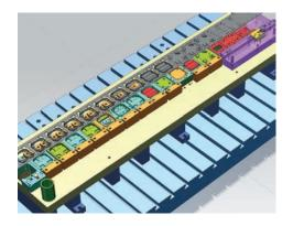
The new knowledge reuse library for standard parts and die bases provides faster lookup and design insertion. Adding a standard part to a design is as easy as drag-and-drop and the library includes the latest available supplier catalog content.
