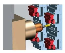
Volume based 2.5 axis milling Traditional 2.5 axis milling is more intuitive and more productive than ever with the new selection approach in NX 8 CAM. Cutting volumes are quickly identified based on floor and wall selections. These floors and walls in combination with the in-process work piece (blank stock) result in volumetric cut regions.
