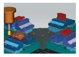
Hole/boss milling Holes and bosses get special handling in NX 8 CAM for optimum milling. Geometry selection supports both manual and feature based operation types.
