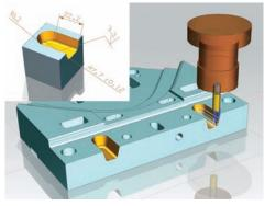
Additionally, with the new Teach Operations function you can easily build up machining process definitions from NX CAM operations and identify process specific parameters such as cutting, noncutting, user-defined events (UDEs), cycles, and cycle parameters, cut levels and KF parameters. Then optionally edit machining rules in the Machining Knowledge Editor (MKE) to make them more general.
