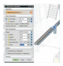
select and place parts based on destination characteristics and run definition, with part search criteria based on defined rules and relationships. The latest release also adds duct size calculators for HVAC ducts based on flow parameters, and a pipe production length checker and calculator that determines shrinkage compensation and the appropriate bend machine.
