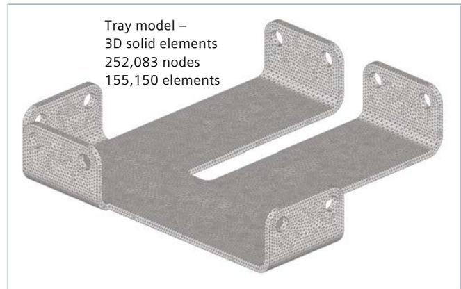
Figure 5: Thin walled model size comparison.
