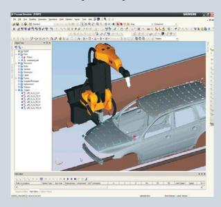
Process Simulate facilitates the design and validation of manufacturing processes in a 3D dynamic environment. Process Simulate is fully integrated
