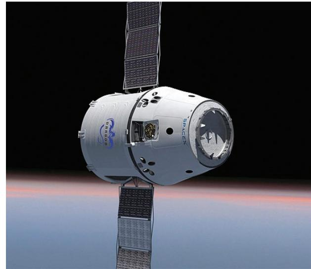
*SpaceX DragonLab is a free-flying, fully recoverable, re-usable spacecraft capable of hosting pressurized and unpressurized payloads. Fibersim is being used to assist with actual fiber placement for the spacecraft's thermal protection system, including the heat shield, exterior panels, insulating layers on the rocket and spacecraft, and several panels around the nose cone and engines. Credit: SpaceX*
